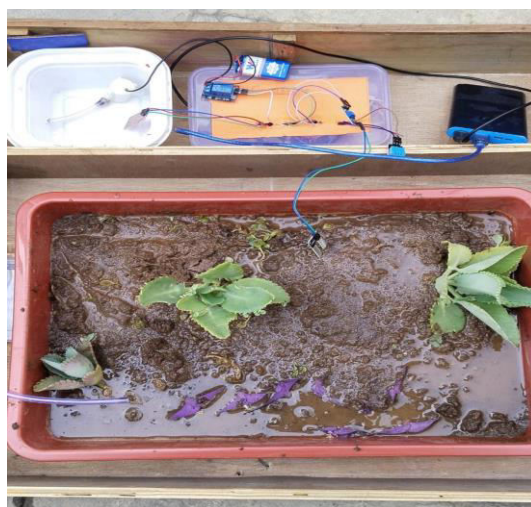
Fig. 2- Sensor's measurement and store the data in the Esp 8266 send the data to web page via Wi-Fi.
