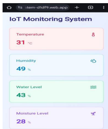
Fig. 3- Output on Web page moisture level less than 40 % motor will turn ON.
